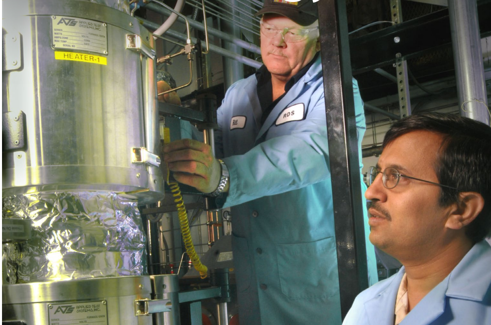
NETL's Dushyant Shekhawat and Bill Grimes are preparing the Catalyst Screening Unit in NETL's Reactor Laboratory for diesel reforming runs.
