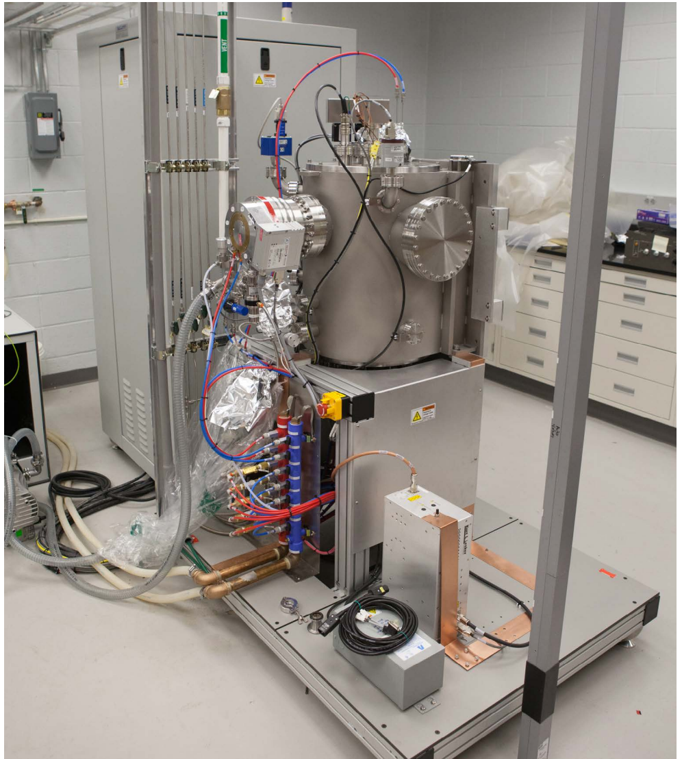
The Kurt J. Lesker Lab 18 Unit is housed in the Pittsburgh Materials Preparation and Characterization Facility and benefits many researchers at NETL, providing precise application of thin films.
