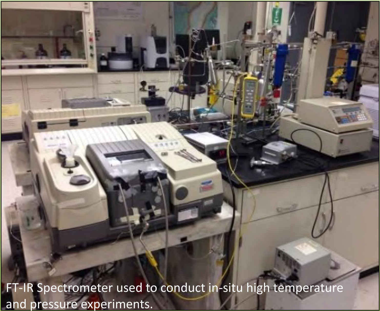
Multi-bounce with sample holder for FT-IR
