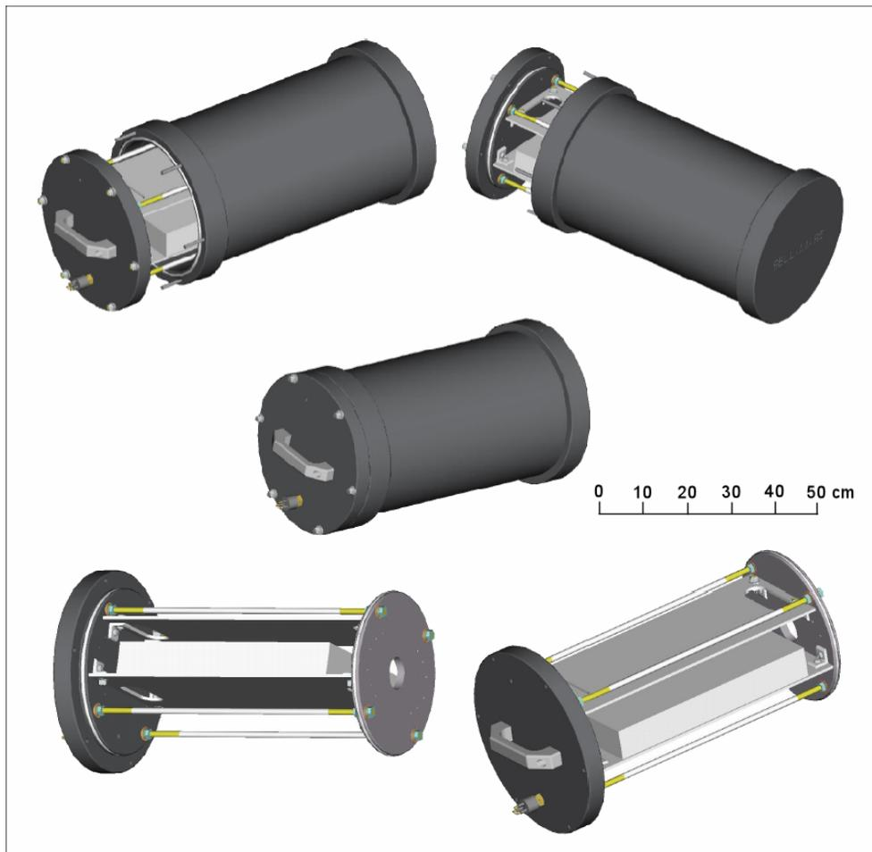
Figure 1. Proposed pressure housing design from Ocean Innovations, LLC., La Jolla, California. The inside diameter is 25.4 cm, length 50.8 cm, hull thickness 1.3 cm. The rectangular box shown in the housing is the approximate maximum dimensions of the AGI 8-channel receiver board. The housing is shown without the penetration through the non-opening end-cap.
