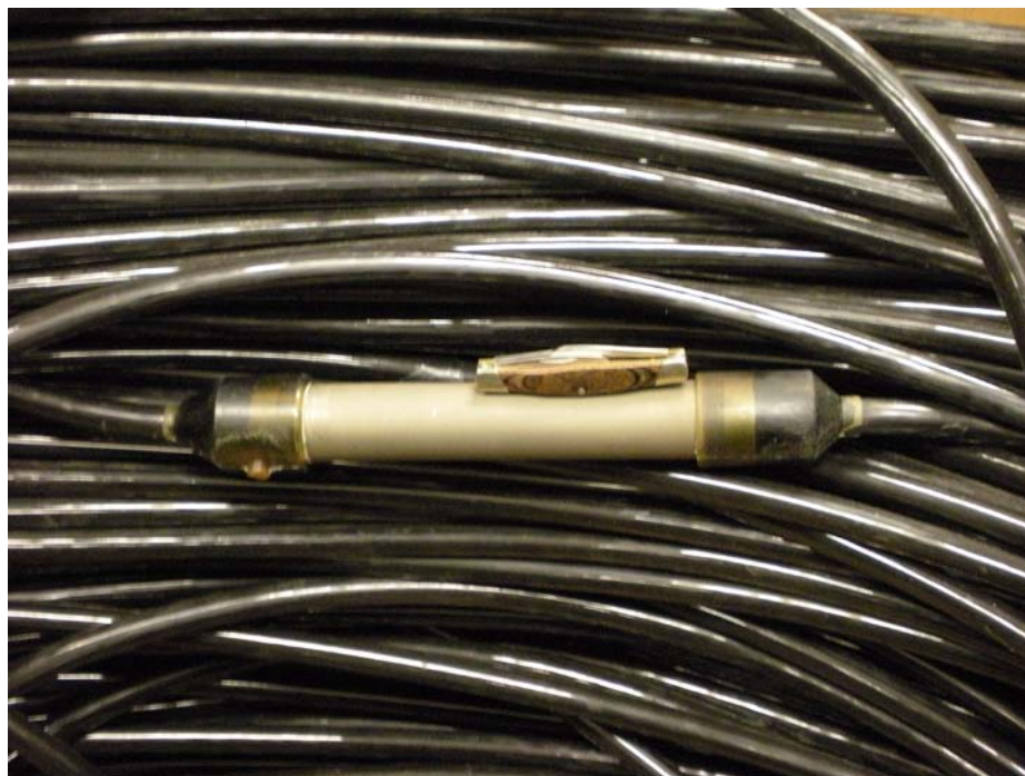
Figure 2.1. Titanium receiver electrode. The new resistivity array for Phase 2 has 10 dedicated receiver electrodes made of titanium and three dedicated source electrodes made of copper. The electrodes were molded into the array at fixed positions, 50 m apart. The electrode shown is a 20 cm-long, titanium receiver electrode, molded into place on the cable.
