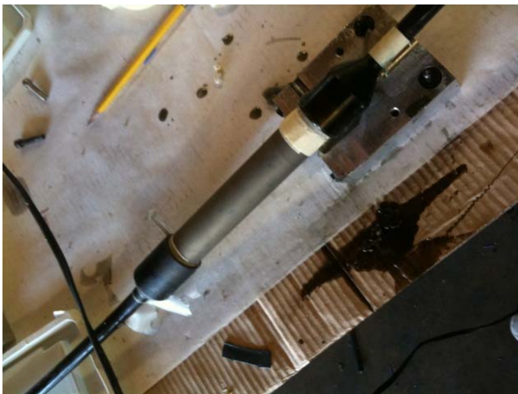
Figure 2.1. Molding of a receiver electrode. The new resistivity array for Phase 2 will have 9 dedicated receiver electrodes made of titanium and two dedicated source electrodes made of copper. The electrodes will be molded into the array at fixed positions, 50 m apart. The electrode shown is a 20 cm-long, titanium receiver electrode, molded into place on the cable.
