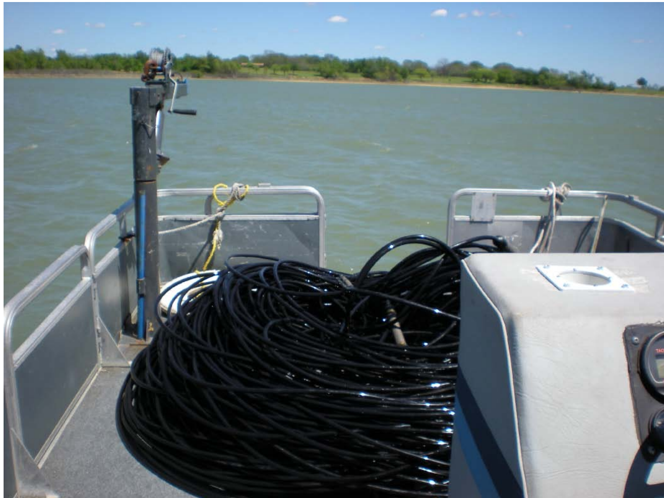
Figure 2.1. Deployment of the seafloor electrode array in Lake Lavon, Texas.
