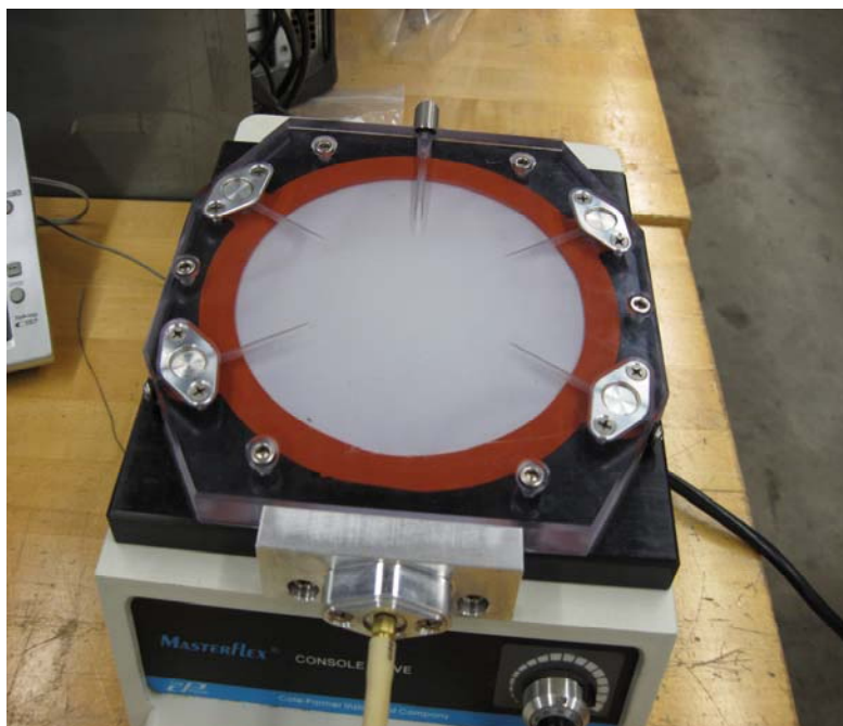
Figure 32. Filter assembly mounted on distilled water pumping station.
