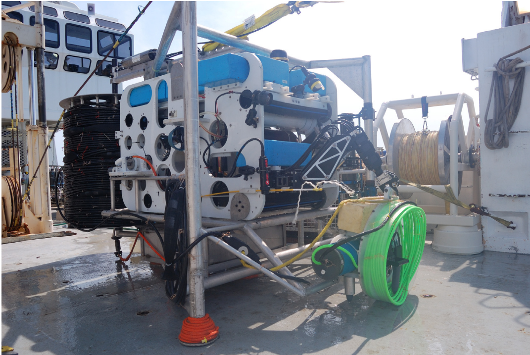
Figure 6. The SSD configured to carry the HLA, DATS and connectors.
