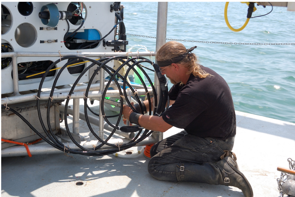
Figure 7. Matt Lowe bands the leading loops of the cable to the SSD so that they ride smoothly to the seafloor, 900m down, ready to begin unspooling.
