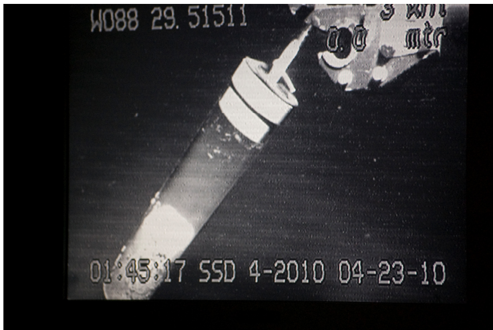
Figure 26. The SSD collecting targeted a push-core.
