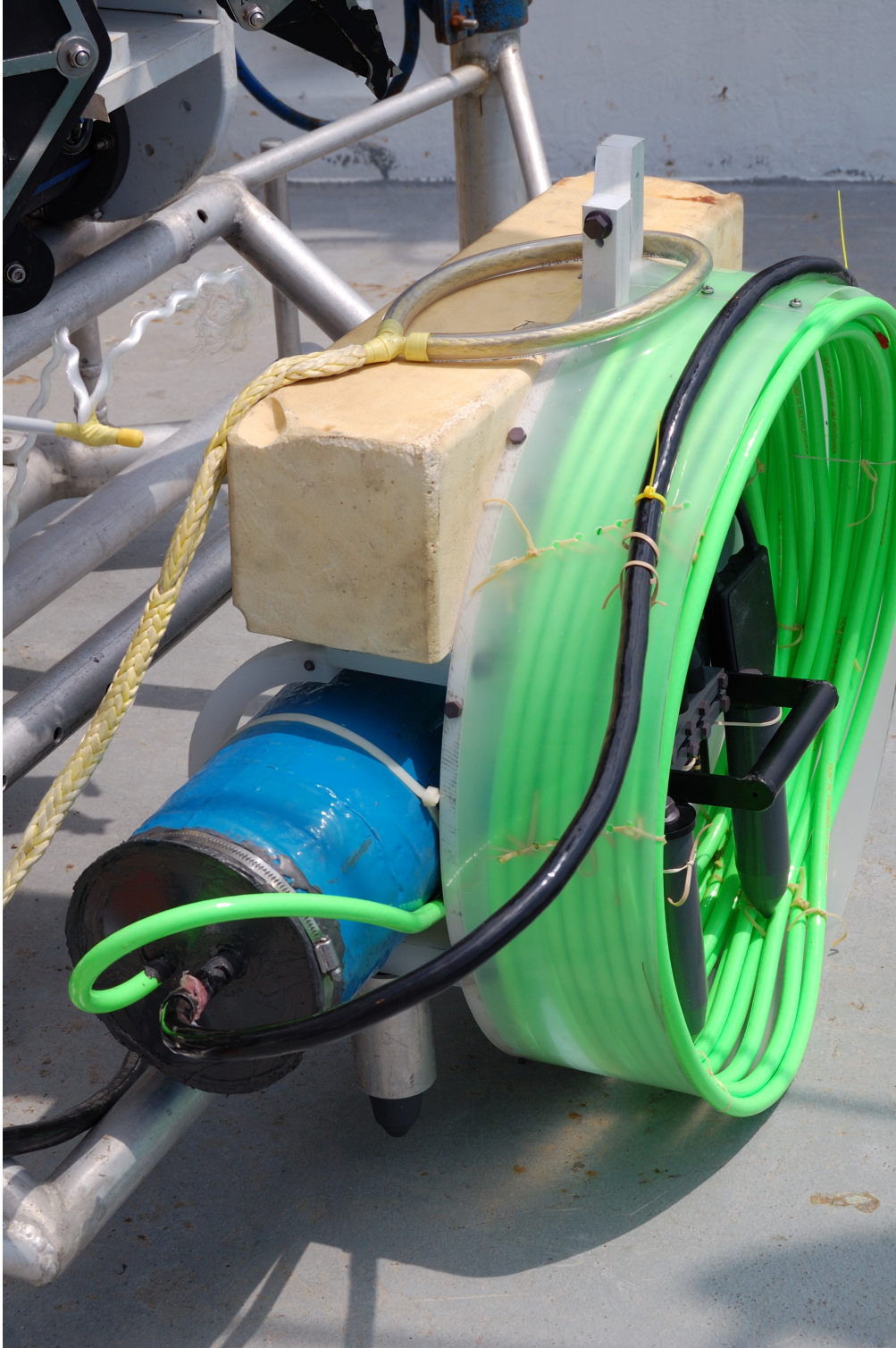
Figure 8. Close-up of the DATS and connectors (to the IDP) ready to ride to the seafloor. The transporter includes the make and break underwater ROV compatible connector which mates the HLA DATS to the IDP.
