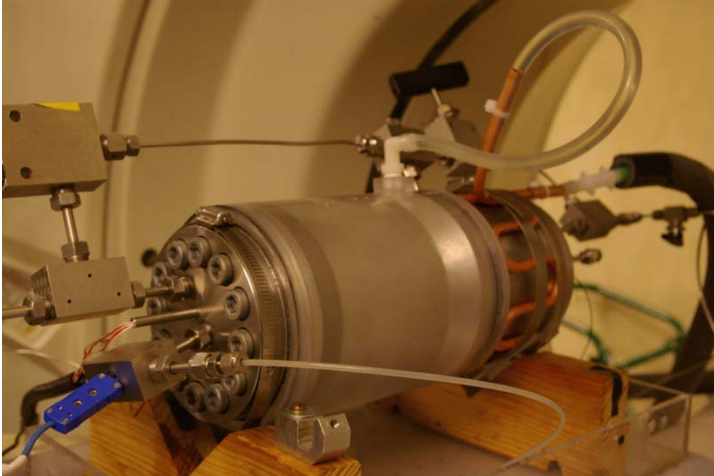
Figure 2-13. Pressure vessel containing sample mounted on x-ray CT scanner.
