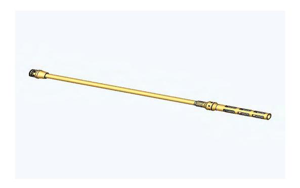
(2) Designed and fabricated two (2) sets of four (4) weight collars (10 feet long). The weight collars served to accommodate the long distance between the reaction point in the ODP BHA, and added weight required to lower the tool through the long drill string.
