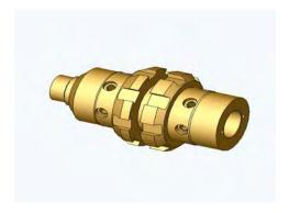
(5) Designed and fabricated adaptors to connect the mechanical pawls to thick wall tube.
