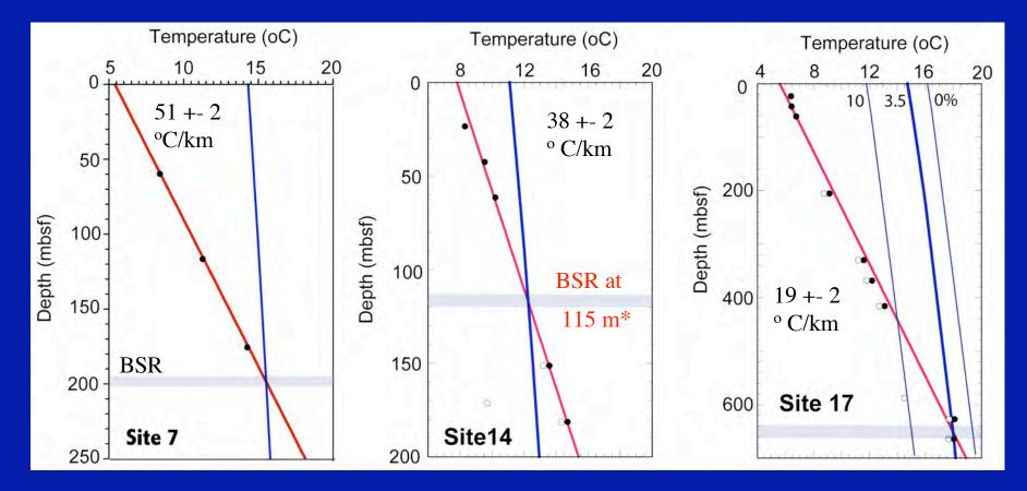
Data generally well fit by a straight line (i.e. a conductive thermal gradient in medium with constant thermal conductivity).
