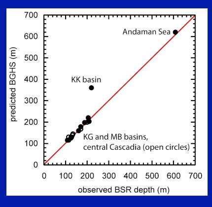
Base of gas hydrate stability predicted by in situ temperature data corresponds closely with observed BSR depth in almost all cases:
