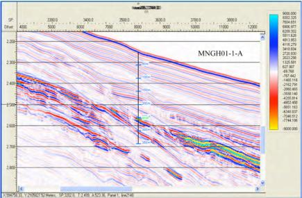
Without drilling constraints, uncertainty in heat flow from BSR is quite large (up to 50%). With drilling to constrain thermal conductivity and depth (velocity), data uncertainties are small ( $\sim$ 5%).
