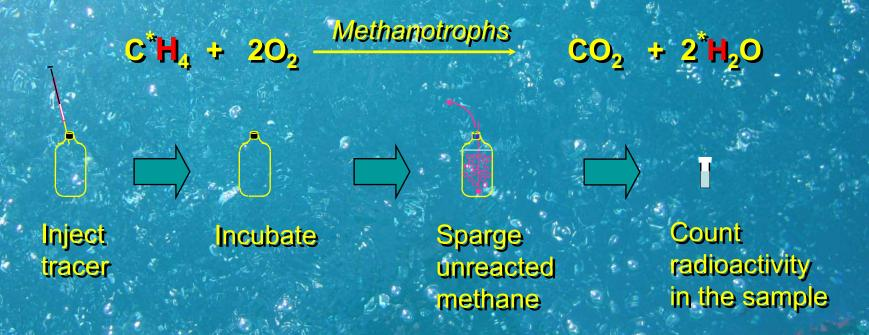
Oxidation rate = Concentration × Fraction oxidized
