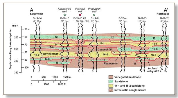
Cross-section through the pilot test area of the Citronelle Field shows the challenge of geologic complexity in fields where CO, flooding is being considered. Well B-19-10 #2 is the CO, injection well.
