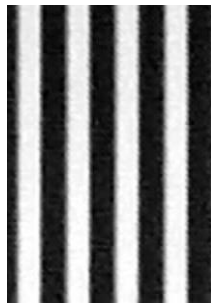
100 MHz: fingerwidth 8 \mu\text{m}
