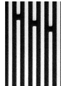
250 MHz: fingerwidth 3 \mu\text{m}
