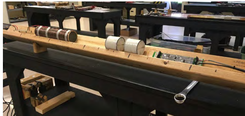
Initial bench testing of TX-RX coil setup
