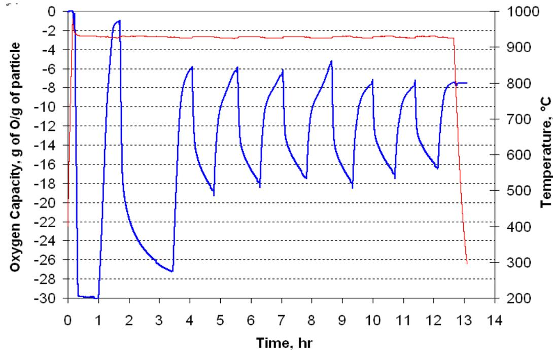
Commercial  $Fe_2O_3$  particles lose reactivity within a few cycles
