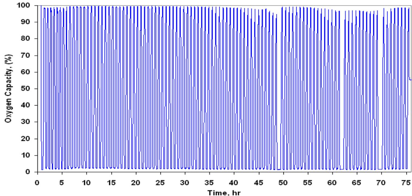
Composite  $Fe_2O_3$  particles sustain multiple redox cycles without significant loss in activity
