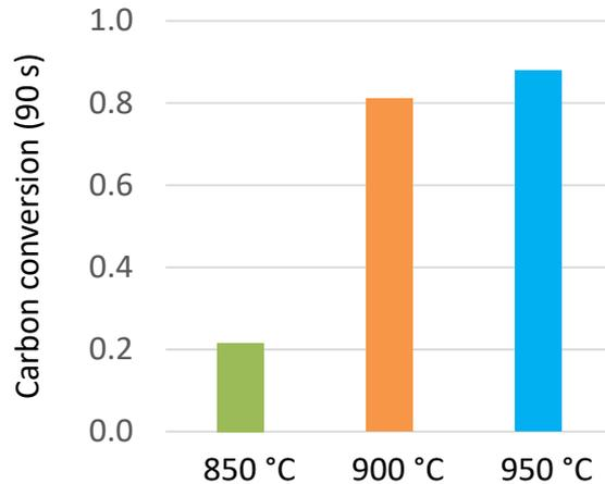
Carbon conversion of char at 90 seconds at 900 C fluidizing in steam.
