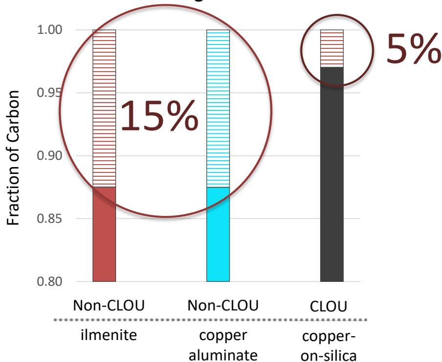
Carbon conversion at 90 seconds of the 400-micron char at 900 C, fluidizing in steam.
