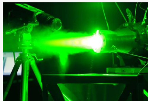
PIV on exit plane of nozzle of the Aerojet RDE
