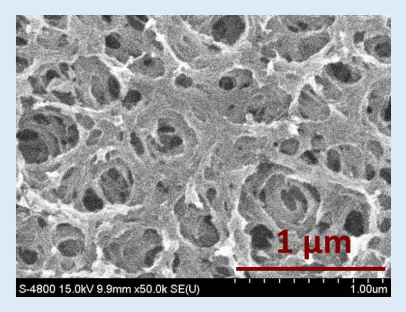
UKy-CAER developed Carbon Xerogel (CX) is a type of mesoporous electrode material CX has an approximate surface area of 150 m<sup>2</sup> g<sup>-1</sup> with a high adsorption capacity towards nitrosamine compounds CX shows excellent chemical stability, conductivity, native ionadsorption capability, and solvent wettability
