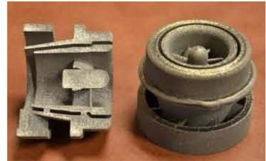
cSETR swirl injector element using additive manufacturing
