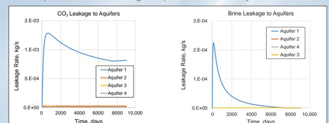
Figure 5. Plots of the results obtained with the Multisegmented Well Model: a) CO<sub>2</sub> leakage to aquifers vs. time and b) brine leakage to aquifers vs. time.
