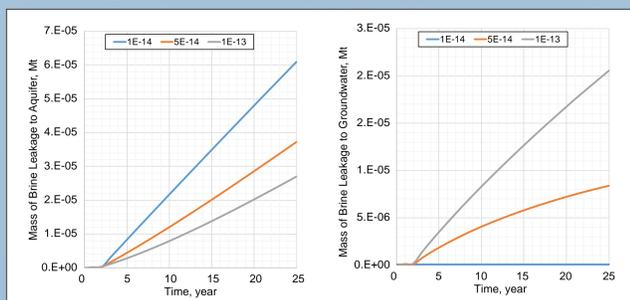
Figure 7. Sensitivity analysis of wellbore cement permeability on brine leakage: a) rate of brine leakage to the shallow aquifer and b) total mass of brine leakage to the groundwater.
