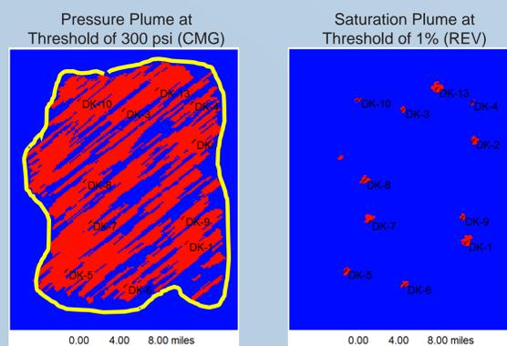
Figure 3. Maps showing top view (XY plane) of a) the pressure plume threshold (left) and b) the CO<sub>2</sub> plume threshold (right). Results correspond to Geological Realization 1 (P10) after 25 years of injection.
