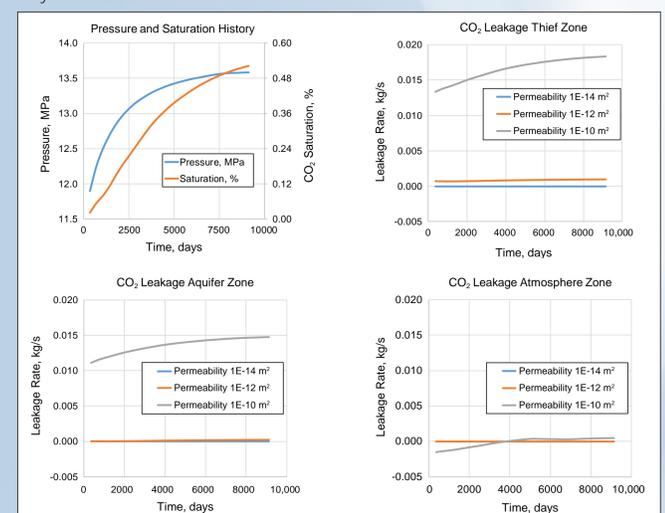
Figure 4. Cemented Wellbore Model inputs and results: a) pressure and saturation history from Computer Modelling Group Ltd. (CMG) results, b) CO<sub>2</sub> leakage rate to the Thief Zone, c) CO<sub>2</sub> leakage rate to the Aquifer Zone, and d) CO<sub>2</sub> leakage rate to the Atmosphere Zone. Note that 1 kg/s is equivalent to 86.4 Mt/day.
