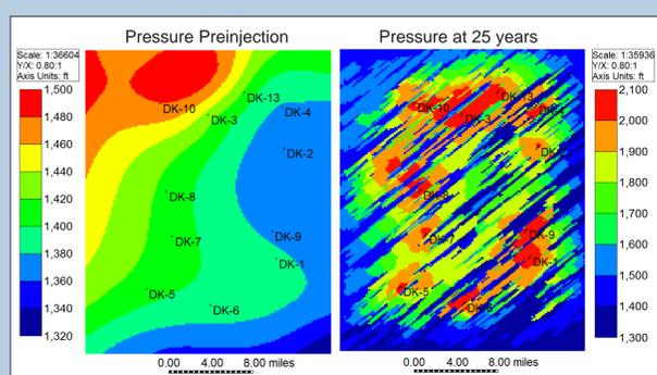
Figure 1. Maps showing a top view (XY plane) of the pressure plume for Geological Realization 1 (P10) at a) before starting the CO<sub>2</sub> injection (left) and b) after 25 years of injection (right).
