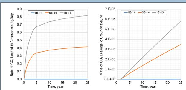
Figure 6. Sensitivity analysis of wellbore cement permeability on CO<sub>2</sub> leakage: a) rate of CO<sub>2</sub> leakage to atmosphere and b) total mass of CO<sub>2</sub> leakage to the groundwater.
