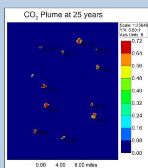
Figure 2. Maps showing a top view (XY plane) of the CO<sub>2</sub> saturation plume for Geological Realization 1 (P10) after 25 years of injection.
