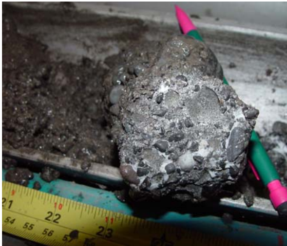
Figure 4. Photograph of a gas-hydrate-bearing rock core from the Mallik 5L-38 Gas Hydrate Research Well. Note that the gas hydrate is the white material filling the void spaces in this conglomerate (photo courtesy of the Mallik 2002 Gas Hydrate Production Research Well Program).
