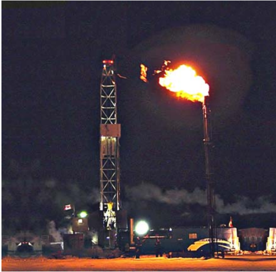
Figure 5. Photograph of the gas flare from the thermal gas hydrate production test in the Mallik 5L-38 Gas Hydrate Research Well (photo courtesy of the Mallik 2002 Gas Hydrate Production Research Well Program).
