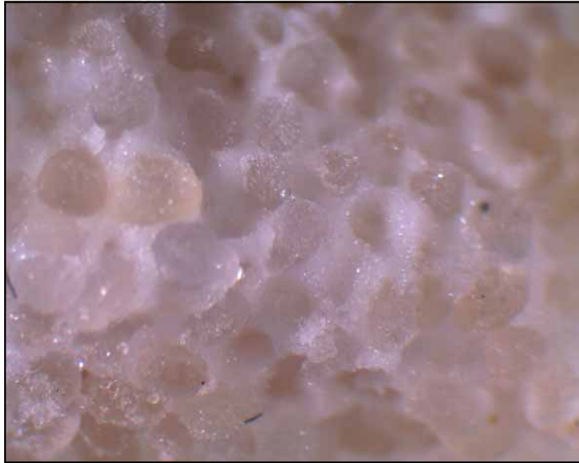
• Photo of sand sample extracted from a column after being injected with a • microemulsion of CO 2 and water to extract methane from methane hydrate.
