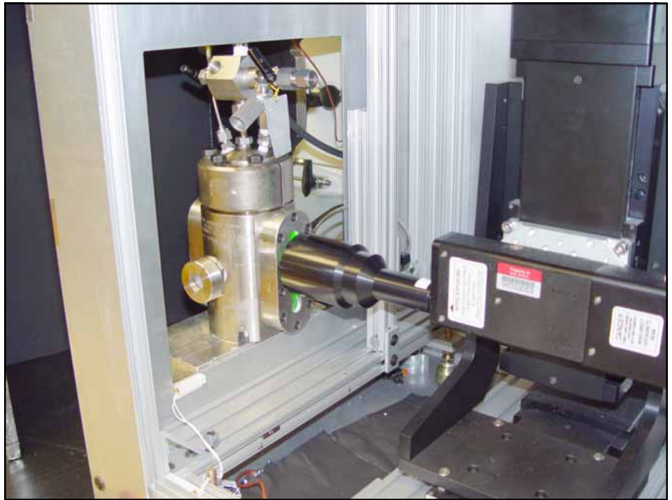
Scanning Laser Raman LIDAR (Light Detection And Ranging) System and pressure cell equipped with a sapphire window
