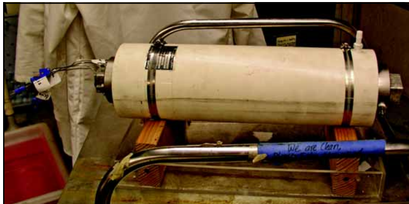
Core-scale pressure vessel in a water jacket for temperature control. Thermocouples extend from the left side.
