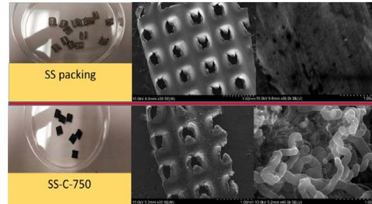
Photograph and SEM pictures of as-received and carbon-coated stainless steel packings
