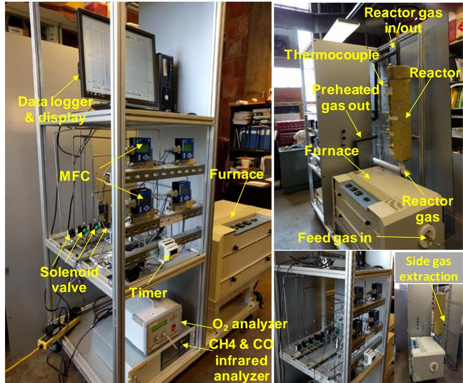
□ RFFB system recently built for bench-scale testing of selected catalysts:
