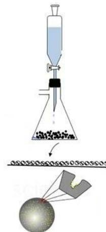
Metal precursor solution to wet particles and fill pores
