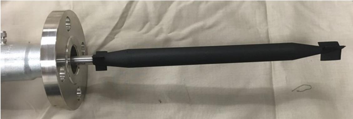
**Figure 72: Subsonic ICES 3D Printed Centerbody**
