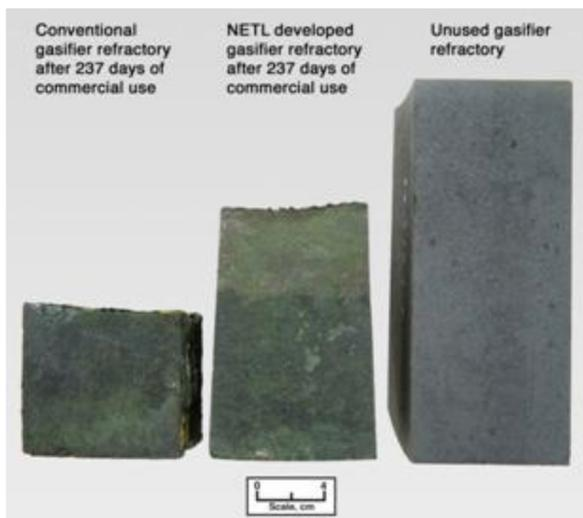
Comparison of conventional refractory (far left) and NETL-developed high-chrome oxide refractory (middle) materials removed from a gasifier using coal as a carbon feedstock after 237 days of service. An unused refractory (far right) is included for comparison. Note that less material is removed from the NETL developed material, which would signify longer service life.
