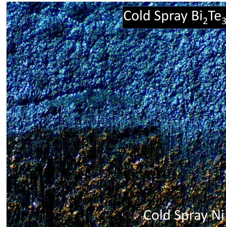
Multi-layer structures show good interfaces
