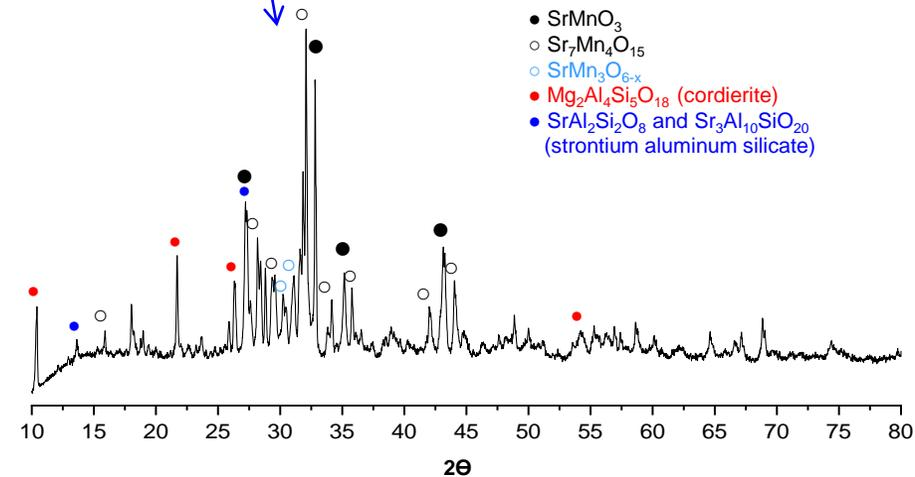
Fabrication of SMO getter composed of  $\text{SrMnO}_3$  and  $\text{Sr}_7\text{Mn}_4\text{O}_{15}$
