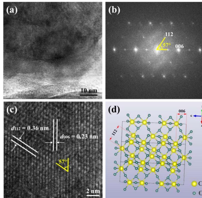
(a) TEM image of region of the chromium deposition taken along [110], (b) The corresponding FFT pattern (c) HRTEM image of the crystalline and (d) the atomic model illustrated.
