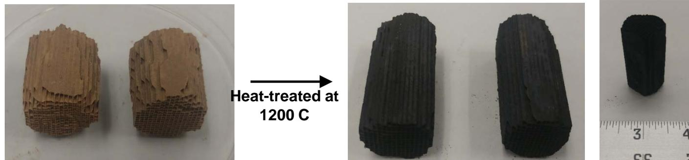
Cordierite substrate coated with the suspension
