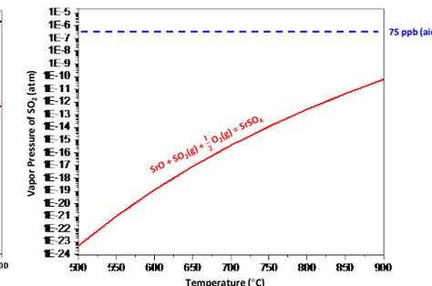
Based on thermodynamic calculations, it is assumed that SrO is capable of absorb Cr vapor (CrO<sub>2</sub>(OH)<sub>2</sub>(g)) and SO<sub>2</sub>(g).
