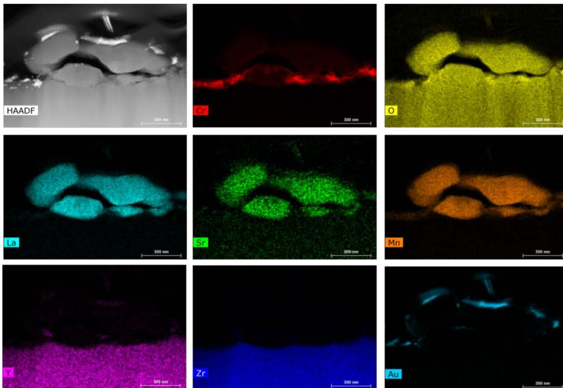
Cross sectional FIB-STEM micrograph and mapping of LSM/YSZ interface after Cr poisoning at 650°C
