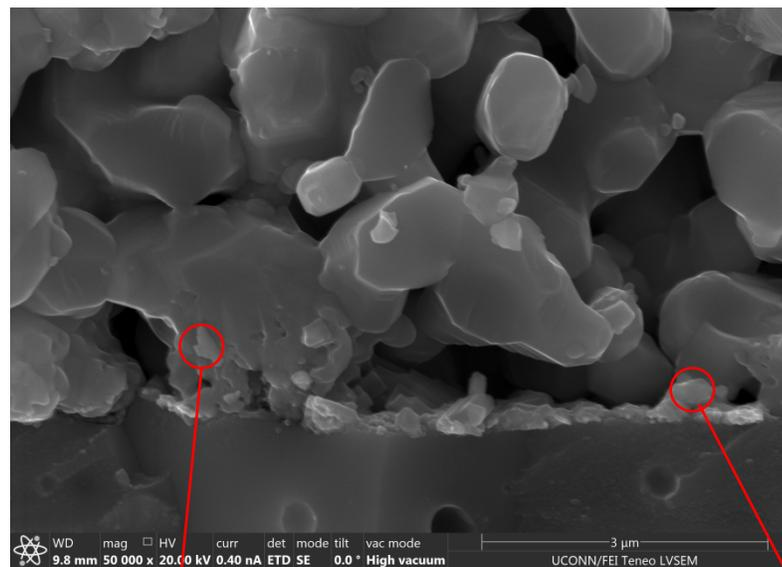
Sulfur elements are also deposited in the interface between LSM and YSZ.
