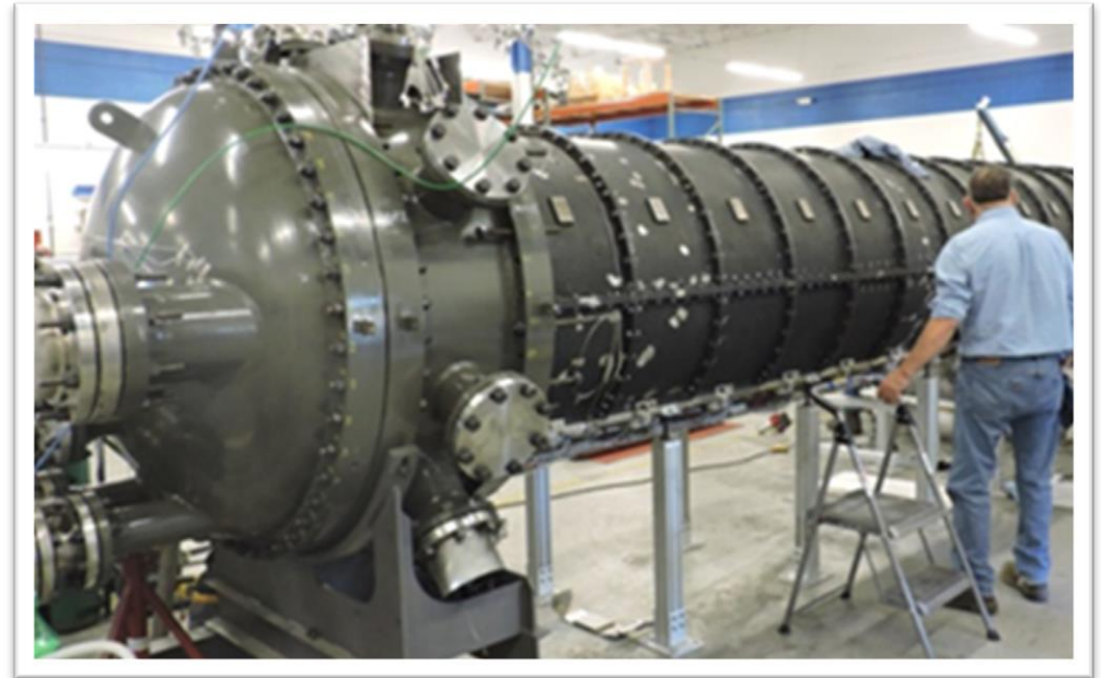
Blocks Assembled into Fuel Cell Vessel
