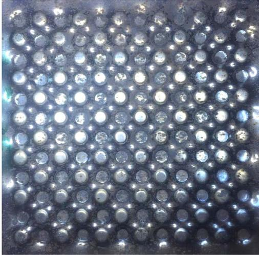
Interconnect with 2 mm in height after firing under load at 800 °C for 5 hours
