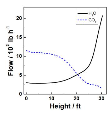
Temperature (left) and flow (right) conditions inside a stripping column. Towards the top of the column, the temperature will rise and significant energy will be expended to vaporize water (lower  $CO_2/H_2O$  ratio).
