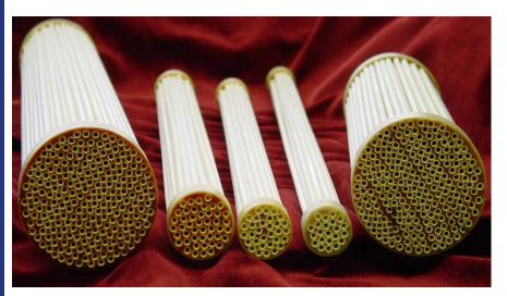
Zeolite Y membrane can stably dewater amine process streams for extended time periods without fouling
