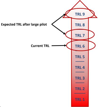
1. Columns expected to achieve TRL 9 based on Linde related experience in building up to  $\sim$  12 m diameter columns for other commercial applications.
