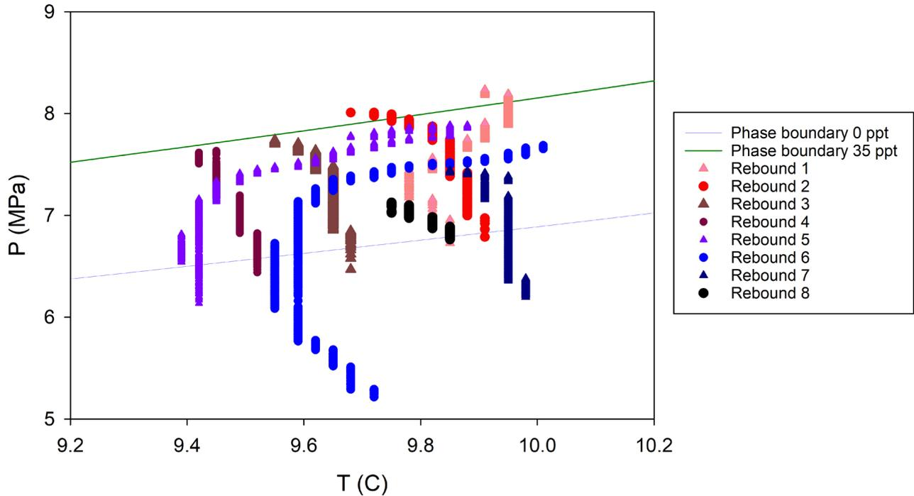
**Figure 7.2.** Pressure versus temperature for each of the pressure rebounds in H002-04CS-1. Shown with the methane hydrate phase boundary for fresh water (0% NaCl) and seawater (3.5 wt% NaCl). During shorter shut in periods (several hours or less) the temperature adjacent to the sample continues to cool over several hours as the pressure rises. During longer shut-in periods the temperature begins to recover and increase in the sample.
