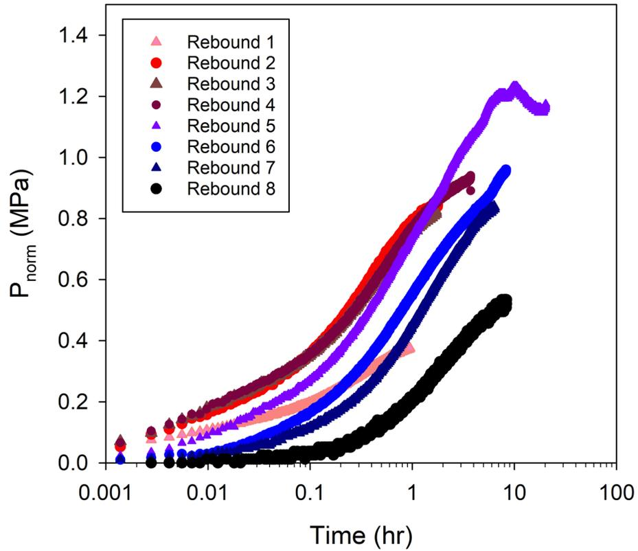
**Figure 7.1.** Pressure rebounds (normalized to the drop in pressure during each gas release) versus the log of time observed in between degassing steps for natural hydrate sample H002-04CS-1. The shape of the curve shows a slower increase in pressure during dissociation as more of the hydrate has been dissociated.
