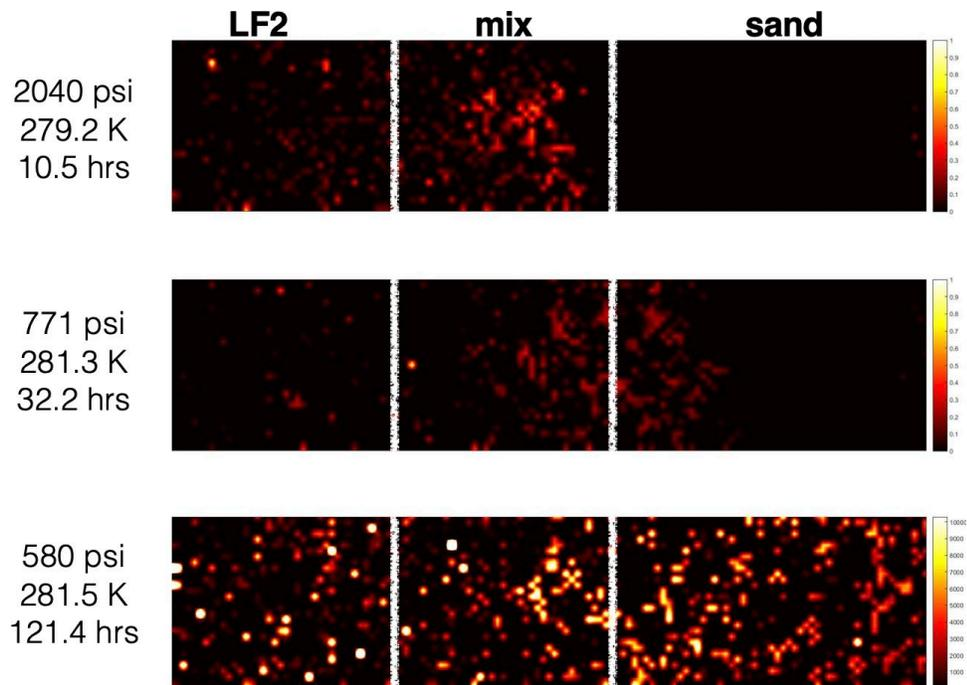
**Figure 9.3.** Methane vapor Raman 2D mapping during methane hydrate dissociation in experiment RH010. The mapping was acquired at the same position as Figure 9.2. Higher intensity (yellow-white color) indicates higher methane vapor presence in the pore spaces.
