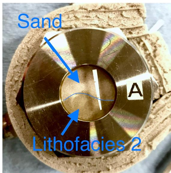
**Figure 9.1.** Photo of 2 kinds of dry sediments loaded in the Raman chamber prior to hydrate formation: sandy silt from core GC955-H005-06FB-2 (Lithofacies 2) and natural
