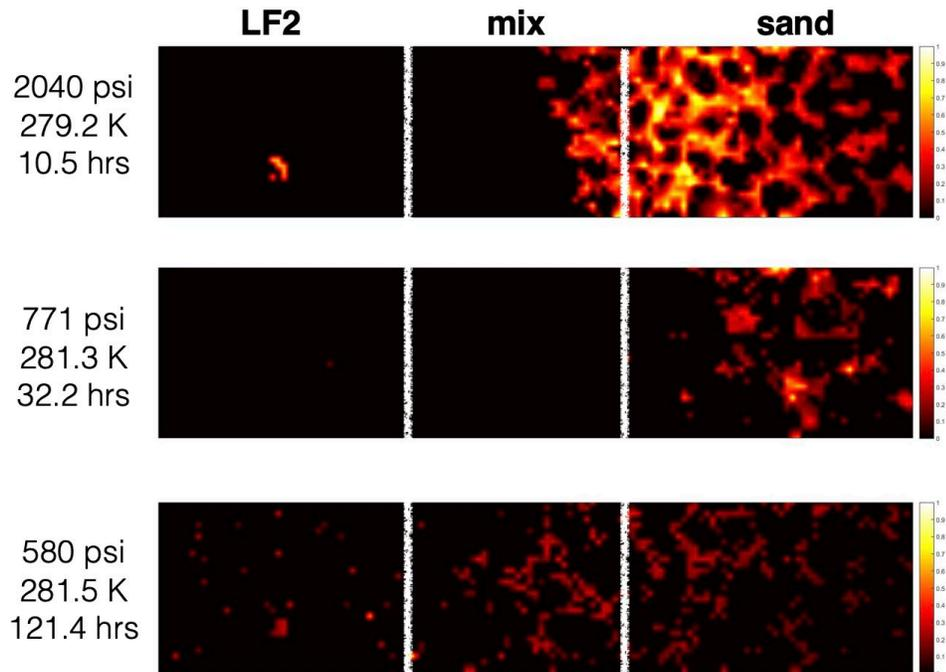
**Figure 9.2.** Methane hydrate Raman 2D mapping during methane hydrate dissociation in experiment RH010. The mapping was conducted near the boundary of lithofacies 2 (LF2) and sand. Materials and fluids can flow freely across LF2, mixture (mix), and sand layers. Higher intensity (yellow-white color) indicates higher methane hydrate concentration in pore spaces.
