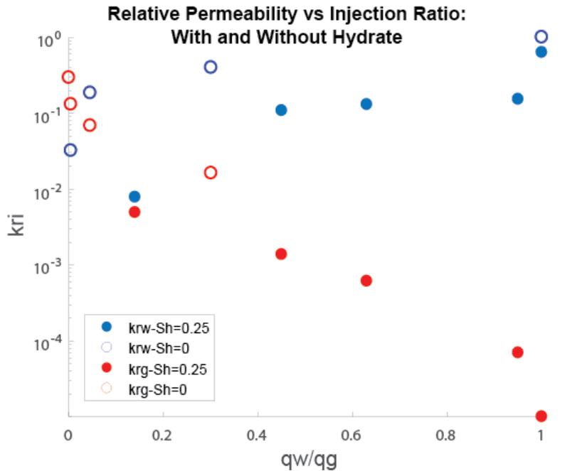
**Figure 6.2.** Comparison of relative permeability data with and without hydrate. Filled circles: data at 25% hydrate saturation. Open circles: data at 0% hydrate saturation.
