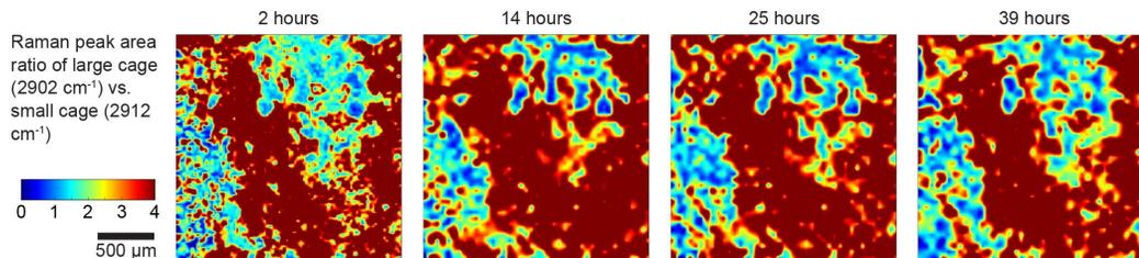
**Figure 9.4.** Raman 2D mapping of spatial and temporal distributions of methane hydrate large-peak to small-peak area ratios. The spatial heterogeneity of hydrate contents and structures from 2-D Raman mappings. Four columns of data are collected at different times after the initial methane hydrate formation. 2D Raman delineate the spatial distributions of methane hydrate large-to-small-cage ratios over time.
