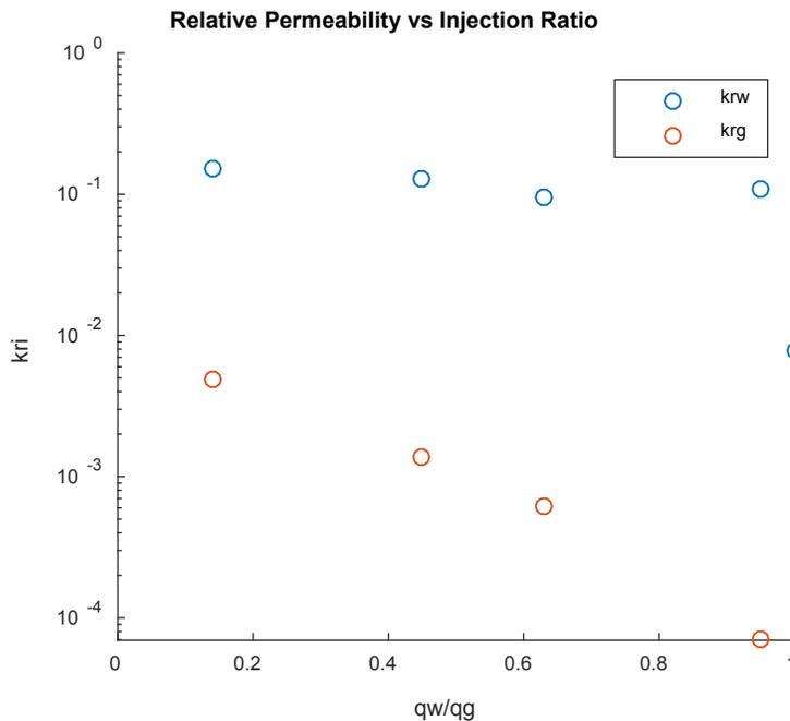
**Figure 6.1.** Relative permeability to brine ( $k_{rw}$ ) and gas ( $k_{rg}$ ) for 5 different injection ratios of gas ( $q_g$ ) and brine ( $q_w$ ).
