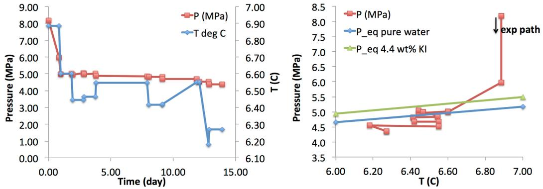
**Figure 8.1.** Pressure-temperature path during dissociation of methane hydrate in a sand-pack.
