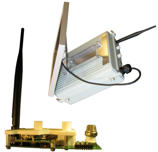
Figure 1. The sensor board selected (capable for use in detecting both CH 4 and CO 2 ) and the ruggedized case to be mounted as part of the UAV platform.
