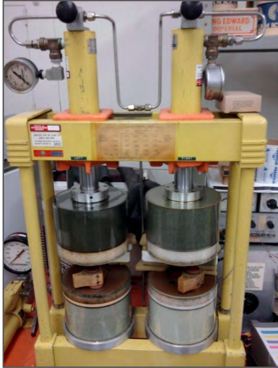
Figure 1. The SMU Geothermal Laboratory divided-bar thermal conductivity measurement apparatus. Samples are placed in between the press where the wooden blocks are located in the picture. The upper unit is heated and the lower unit cooled with constant bath water. The amount of heat/cold that is transferred into the rock is measured by this process and is compared to standard samples to calculate an absolute thermal conductivity.
