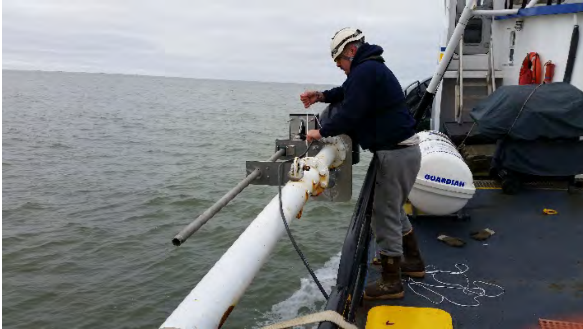
Figure 15: Jim Wells, the Bosun, Securing the 12/200 kHz Knudsen Chirp system to pole on the port beam. This pole was then lowered into the water, where the chirp system could listen in passive mode to the heat flow probe transmitting temperature, location, and tilt information via different pinger signals.
