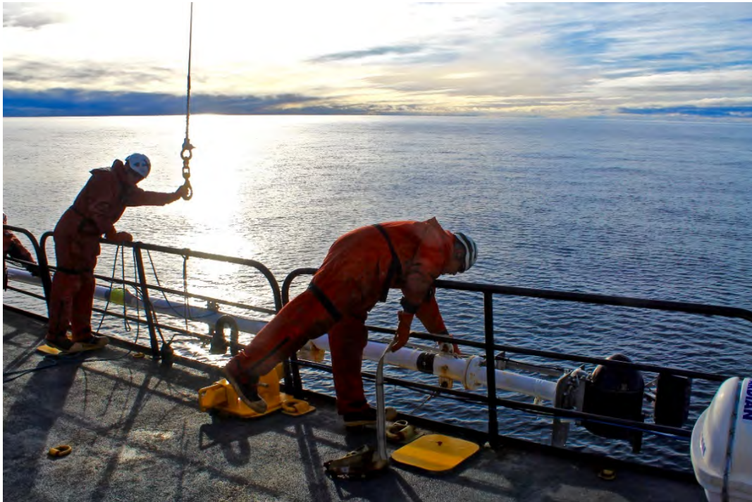
Figure 8: The boom is mounted to the ship's port side during transit, 19 inches away from the side of the deck.
