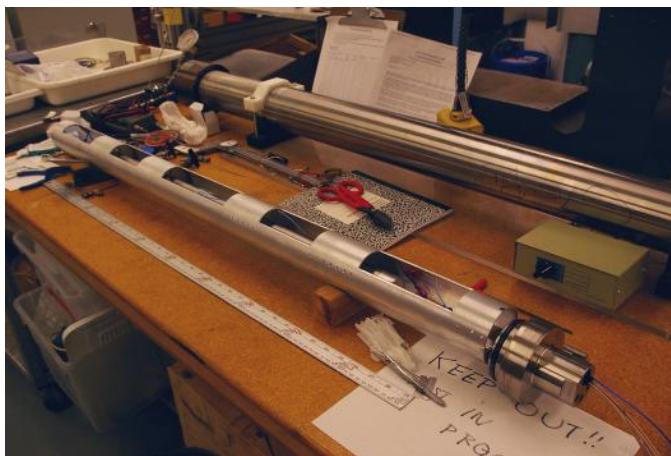
(a) Gas confining cell (top right) and a suspension cage (front) housing the sample-bar assembly
