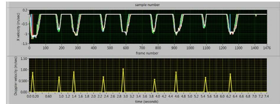
Microwave sensor detects mean particle velocities in L-valve (cold flow testing)
