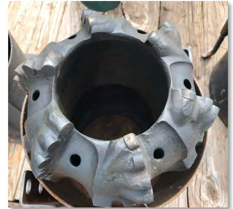
face discharge, low invasion core bit with a tapered face
