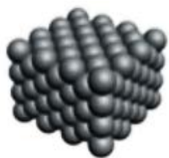
3D opal template (200 nm PMMA colloids on substrate)
