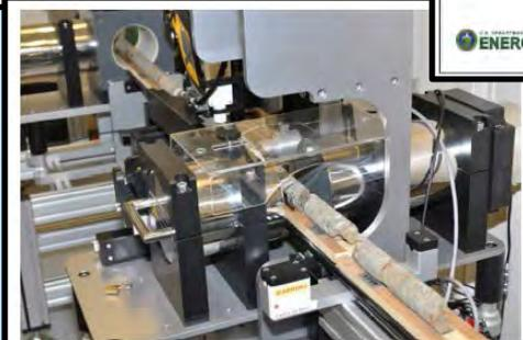
Figure 9. Multi-sensor core logging unit.
