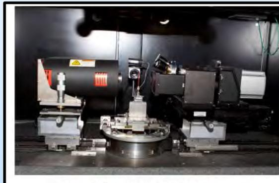
Figure 7. ZEISS Xradia Micro-CT scanner
