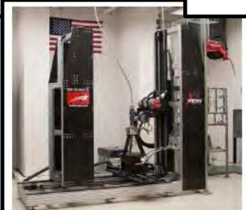
Figure 4. North Star Imaging M-5000 industrial CT scanner.
