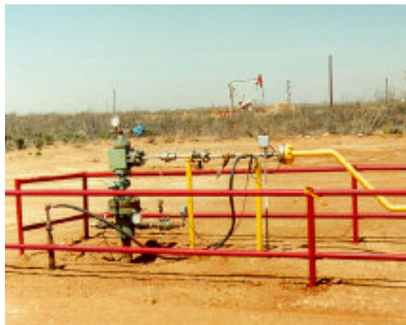
CO 2 injection well, with a pumpjack in the background, part of a CO 2 flood pilot project operated by Advanced Reservoir Technologies Inc. under subcontract from Occidental USA Inc. in Oxy's West Welch Unit in the Permian Basin of West Texas
