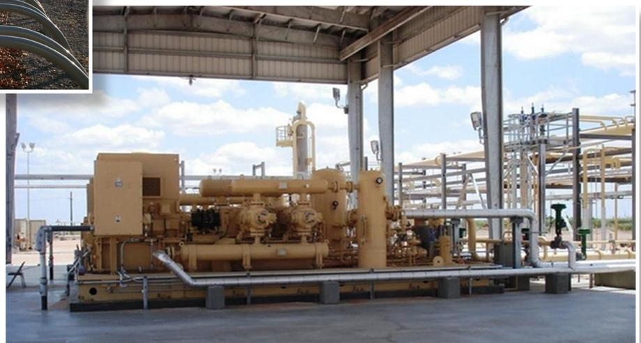
*Compressor for compressing gas prior to re-injection*
