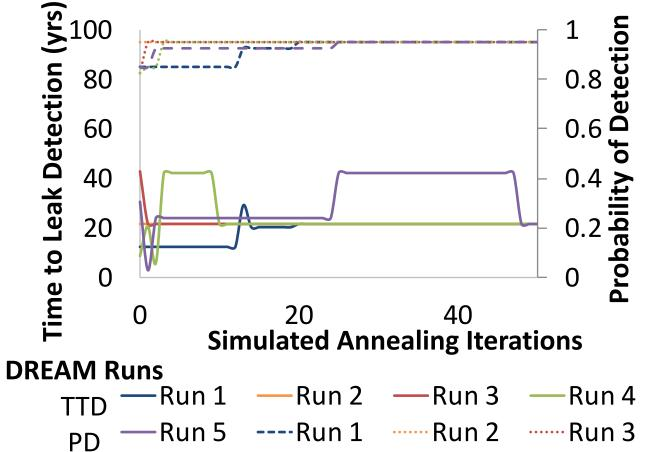
While this data demonstrates the DREAM/ERT sensor placement algorithm, leaked volumes were small relative to realistic ERT detectability.
