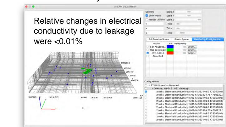
determined for each scenario DREAM used a simulated annealing algorithm to optimize well placements for cross-hole ERT sensors
