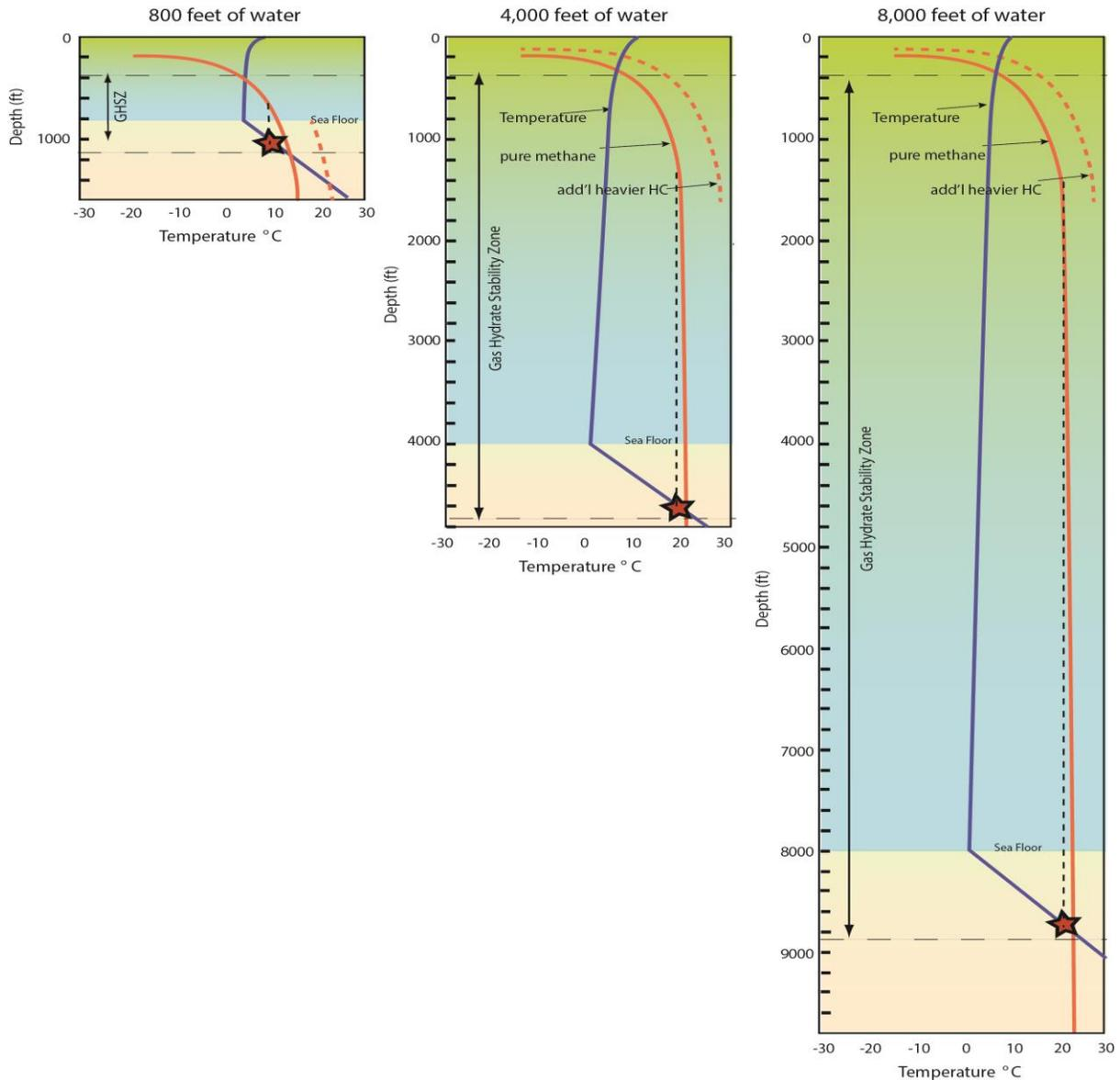
Figure 4: Schematic comparison of gas hydrate reservoir position (red star) relative to schematic stability boundaries (red curves) for various water depths. At great water depths, substantial pressure reduction (dashed black line) is required to initiate dissociation.
