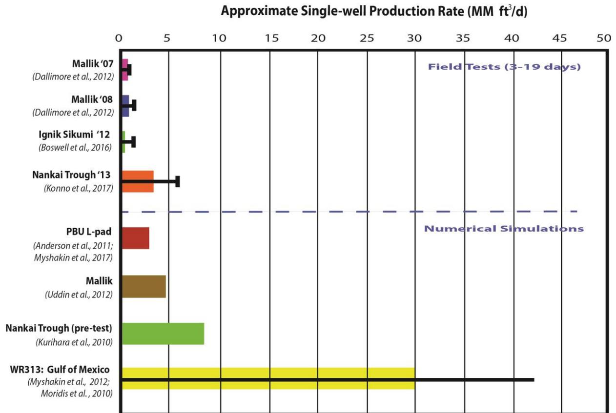
Figure 1: Top: Observed average and peak (black bar) production rates from gas hydrate field production experiments. Bottom: Peak production rates from numerical simulations of production potential over full potential well life. Black bar at bottom shows peak rates obtainable using deviated well designs. Data from [2,4,8,12,15-20]
