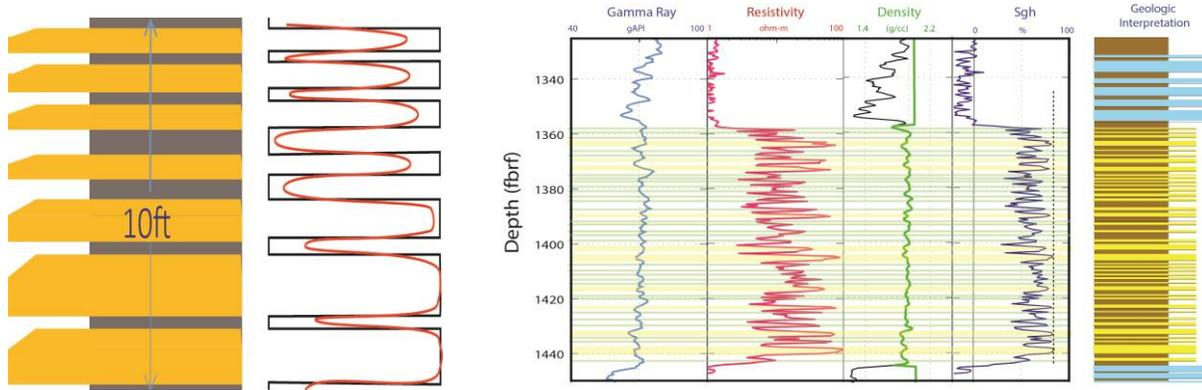
Figure 2. Left: Increased uncertainty in log derived parameters can result where bed thickness is less than vertical log resolution. Red curve is idealized log reading for some generic parameter; the black curve is potential true value of the parameter. The log only reads correct values in beds of sufficient thickness. Right: an example of log data in a thinly-bedded reservoir (Green Canyon block 955; Gulf of Mexico). Modified from [24].
