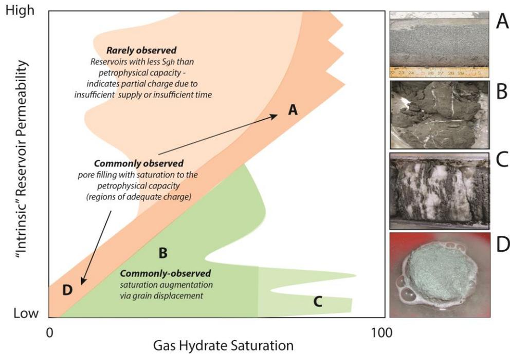
Figure 3. Schematic depiction of observed relationship between gas hydrate saturation ( $S_{gh}$ ) and reservoir quality as represented by intrinsic reservoir permeability. Within pore filling gas hydrates (beige), there is a strong tendency for  $S_{gh}$  to be positively correlated with reservoir quality (modified from [25]).
