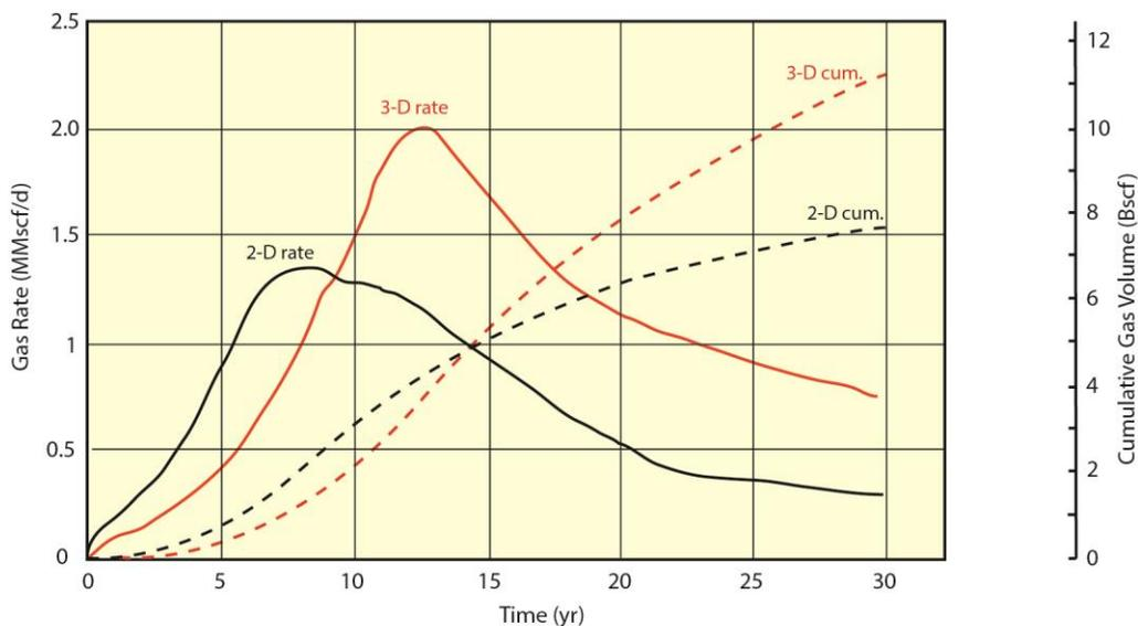
Figure 6. Comparison of 2D and 3D models for a given hydrate reservoir. The models are the same other than the incorporation of modest statistical heterogeneities in reservoir parameters in the 3D case. The results suggest that 3D models are needed even in cases where structural complexities are not expected (from []).
