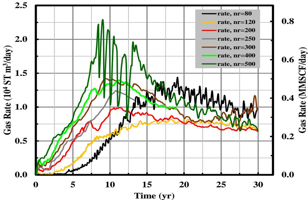
Figure 5. Gas rate profiles using different mesh resolutions. Finer scale grids (higher “nr” values) result in more rapid initiation of production and higher and sooner peak production rates as compared to coarse grids. In all cases, the input geologic/engineering descriptions are identical.
