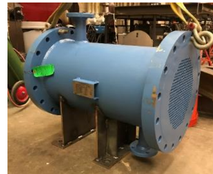
Flue Gas Cooler
