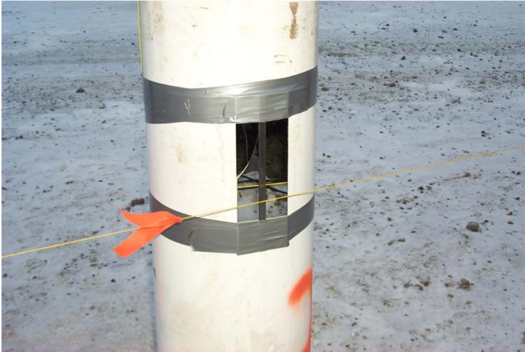
Figure 8 Wire, scale and mirror for measuring displacement
