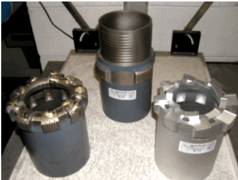
Figure 19. Core Bits Available for the Operation
