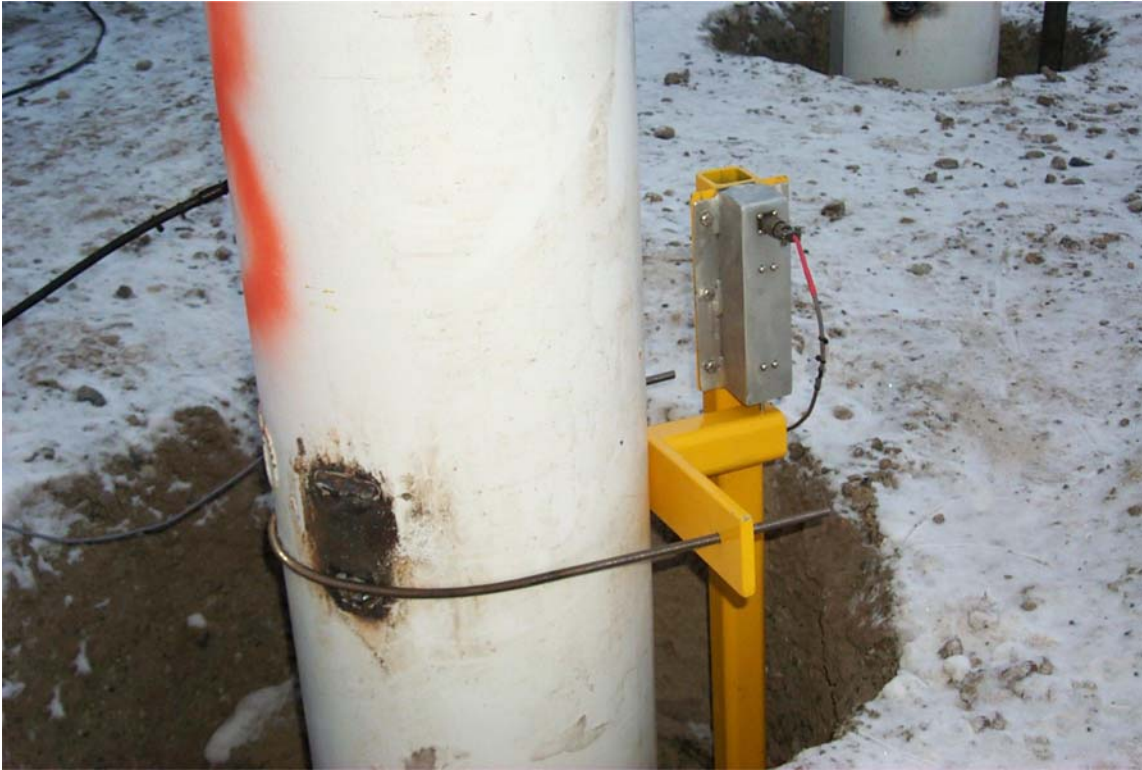
Figure 7 Potentiometer for measuring displacement
