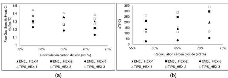
Figure 2: (a) Flue gas specific heat across the heat exchanges for different case studies, (b) Temperature gradient across the heat exchanges for different case studies
