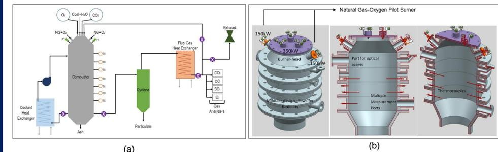
Figure 6: (a) Simplified layout of the combustor system, (b) Proposed 1 MW<sub>th</sub> High Pressure Oxy-Coal combustor concept design
