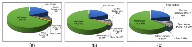
Figure 3: Power distribution of ENEL cycle (a) Case 1, (b) Case 2, (c) Case 3
