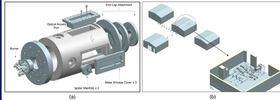
Figure 8: (a) Pilot burner test apparatus (b) Off-campus test facility at Fabens, Texas
