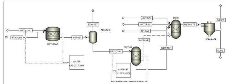
Figure 4: Oxy-coal combustor design in ASPEN Plus®
