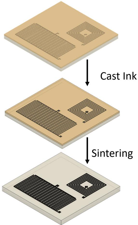
50.8 x 50.8 mm sensor design on Al<sub>2</sub>O<sub>3</sub> substrate.
