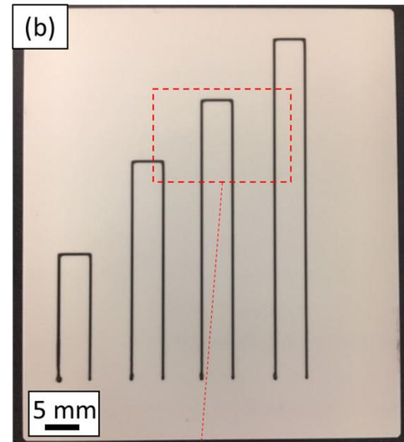
a) Direct ink writing of thermistor array (video). b) Optical image of printed array detailing approximately 400  $\mu\text{m}$  features.
