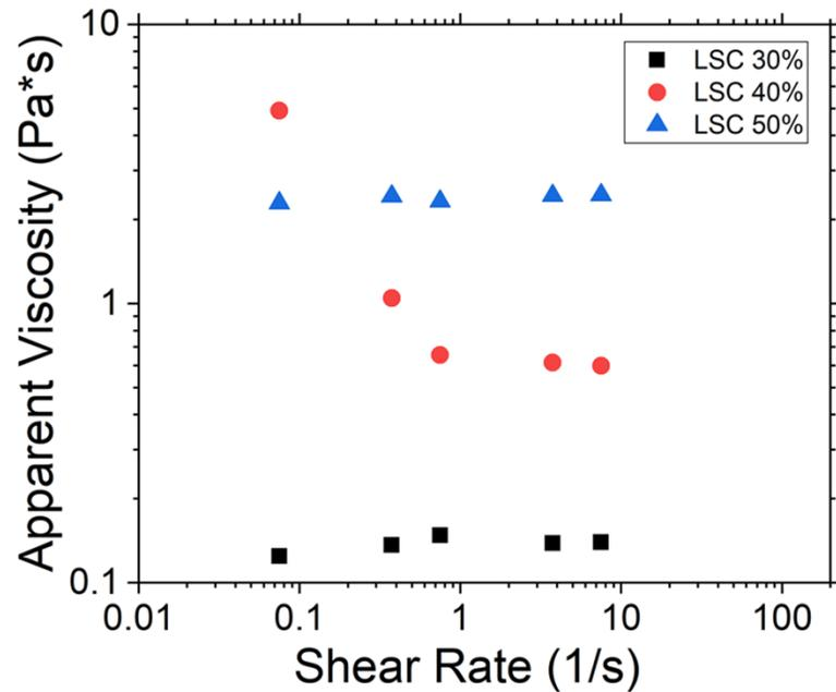
Apparent viscosity vs. shear rate. Percents represent solids loading
