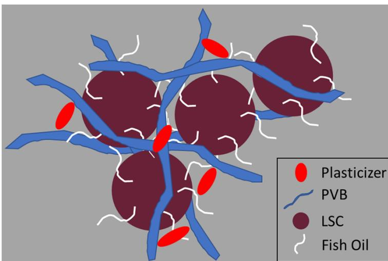
LSC ink schematic. Fish Oil acts as a dispersant, and PVB the matrix material. Ethanol – Toluene cosolvent system (gray) prevents nozzle clogging, while enabling high resolution features.
