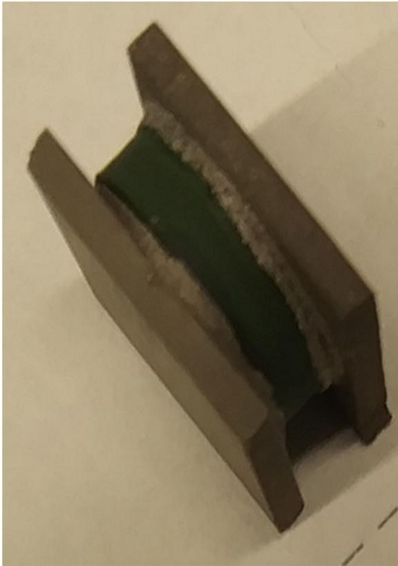
**Ni-LSC-Ni joint brazed with Microbraz 135-S at 1160 °C for 20 minutes in an Argon gas flow rate of 80 SCCM**
