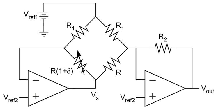
$$V_{out} = V_{ref2} + \frac{R_2}{R_1} \delta (V_{ref1} - V_{ref2})$$
