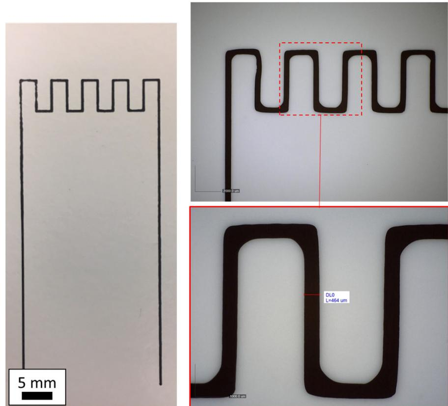
Strain gauge printed using LSC 40% ink from a 100-um nozzle on YSZ tape and alumina. The high wettability allows for strong adhesion, while cosolvent system provides high resolution printing.
