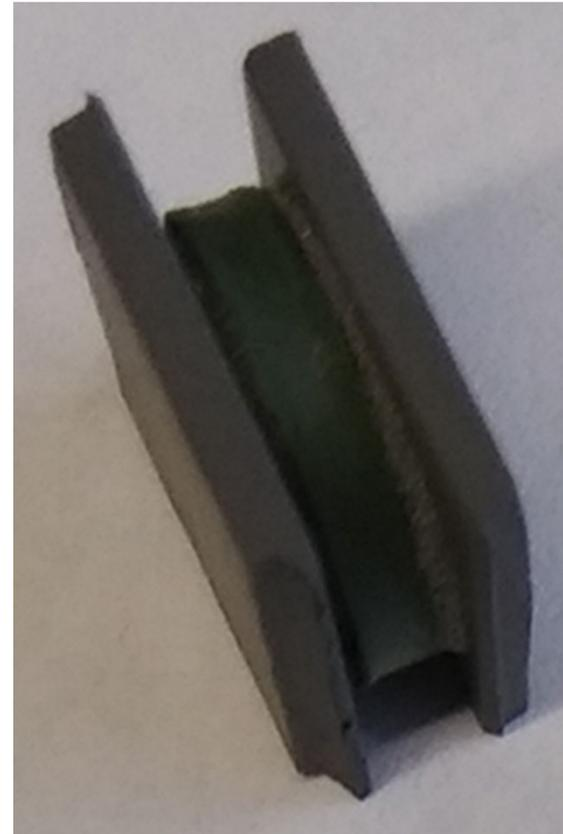
**Ni-LSC-Ni joint brazed with Microbraz 130-S at 1160 °C for 20 minutes in an Argon gas flow rate of 80 SCCM**
