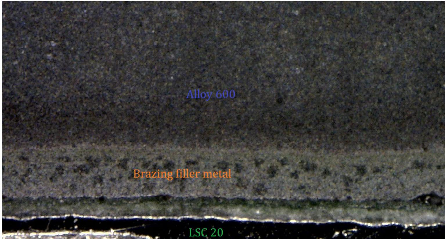
Optical Microscopy at 600x
